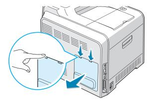
**3** Remove the two screws holding the metal plate in place, and then remove the metal cover, as shown below.
